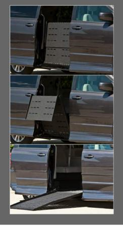
Besides the remote entry, there are also three other power controls inside the vehicle that can operate the mechanism: one by the driver's seat, one by the passenger side door and one in the rear cargo area of the van.
