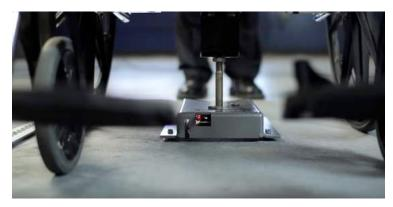
The power tie down (pictured on the left) is the safest, easiest tie down option for wheelchair users. The EZ lock mechanism quickly secures either manual or power wheelchairs in place, so they can remain in place while the vehicle is in motion from point A to point B.
